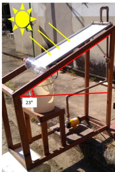
Figure 1. Thin-film fixed-bed reactor used for solar heterogeneous photocatalysis. Source: Authors of the Work.
